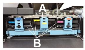
Close Ink Tank Door. Ink colors fill in as Ink Tanks are installed. If ink colors do not fill in after a few seconds, open Ink Tank Door again and reinstall Ink Tank(s).
