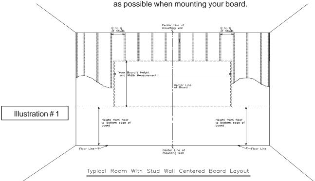
**NOTE:** The proper installation of your board will require at least two people. Tools required: Tape measure, chalkline, electric drill / screwdriver, drill and screwdriver bits, stud finder and level.
