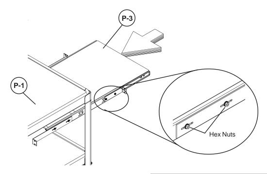
5.) Tilt the Pullout Shelf (P-3) and slide it in the cart. Attach Pullout Shelf (P-3) to Top Shelf (P-1) using 8 screws (A1) and 8 Hex Nuts (B1) as shown in Detail 3A.
