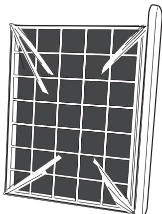
4. Insert Carbon Filter first and then True HEPA Filter.
