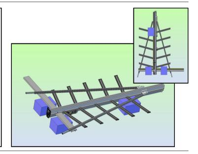
Attach the assembled free standing kit to the back of the machine.
