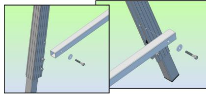
Fix the end of the Stay to the middle of the Cross Bar using a 5mm Allen key and 10mm spanner (wrench).
