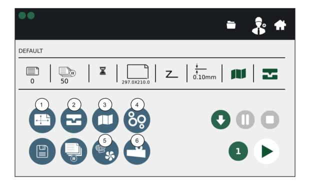
When setting a job on the Pro385, always start with entering the format sizes: leght, width and thickness. Then continue with the adjustment of the crease, fold, roller gaps, fans, choke and delivery module according to the numbering of the picture above.
