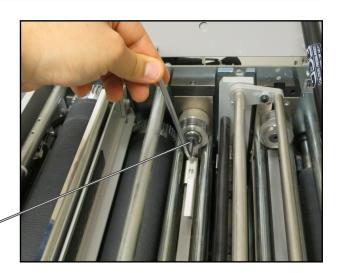
**5** Remove the Sheet Guide Assembly, by pulling upwards on the two flanges (one at each end) as shown [B]
