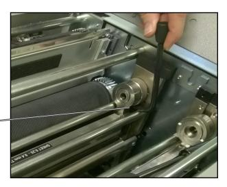
8 Pull the Blade Assembly in the direction shown to unclip and release the Blade Set
