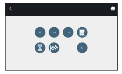
Select batches of 50, 100, 150 sheets. The operator can also enter a custom number of sheets by pressing the "calculator" button.
