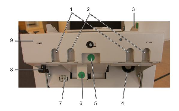
1. Positioning holes, small paper width (310/306:Used for A4/8½" paper widths or sizes nearby. 510: Not used.)
