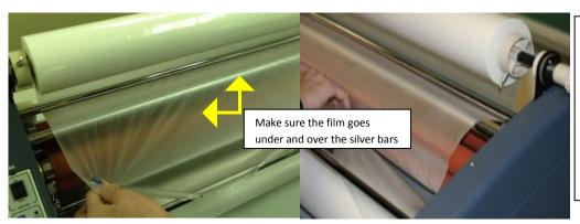
2) Pulling the film through the rollers you need to make sure the film is perfectly aligned at top and bottom. Note: overlap will cause the film to deposit adhesive on the rollers. To thread, you can see the "threading card" that was supplied with the machine.
