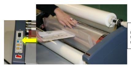
3) You can now power the machine ON by pressing the red power button. Once you insert the threading card in between the rollers and press the ON motor switch the film will thread through the machine.
