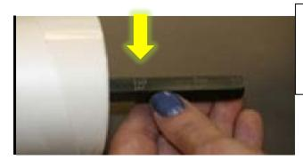
1) Load the film onto rods, by sliding the roll to desired position using the guide marks (25" or 27"), then load the rods onto the laminator. Both top and bottom film rolls should have the dull or adhesive side facing upwards as shown in pictures. Note: you cannot interchange the upper and lower rods
