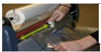
6) You are now ready to laminate! Simply place your desired documents on the feed tray, press the motor ON button, and allow the machine to pull document through. The finished product will come out the back of machine and you can use the attached film slitter to cut at your desired position.
