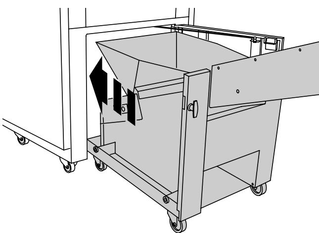
Push back the conveyor belt into the machine.
