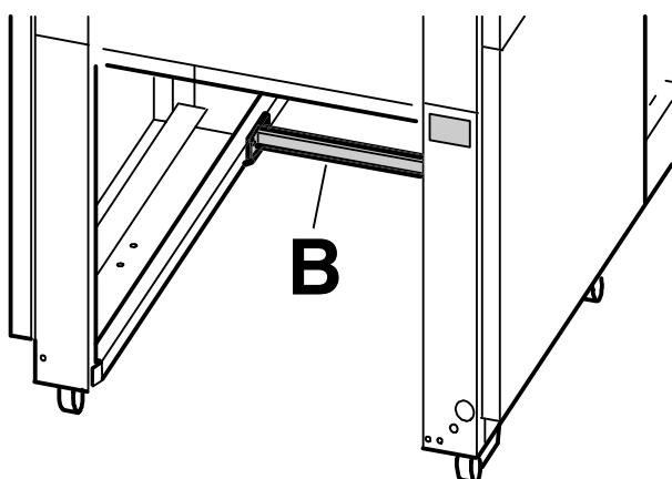
Remove the back transport safety device (**B**).
