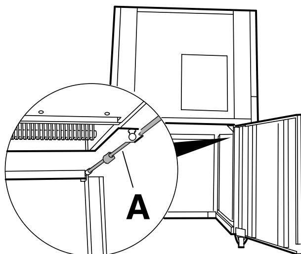
Machine door is difficult to open. → Clean and grease the guiding bar (A). Do not use grease or oil containing resin.
