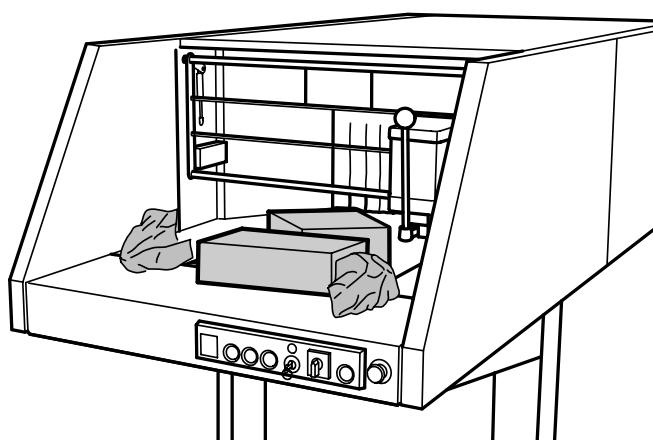
The machine is constructed to shred paper, flat or crumpled, as well as cardboard boxes including staples.
