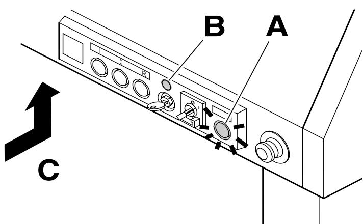
Yellow pilot light (A) illuminates, green light (B) is out → Conveyor belt is overloaded.
