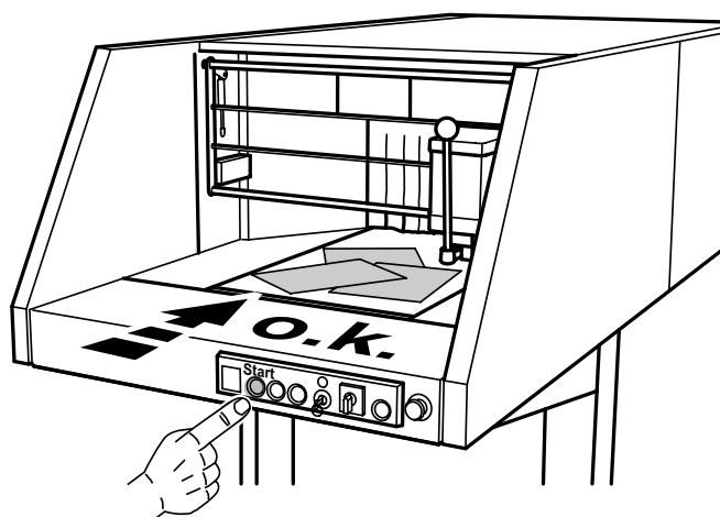
**Check the direction of the conveyor belt.
