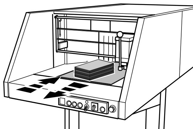
If this capacity is still not powerful enough the machine will reverse shortly and then return to "forwards mode". This is repeated until all material is completely destroyed.
