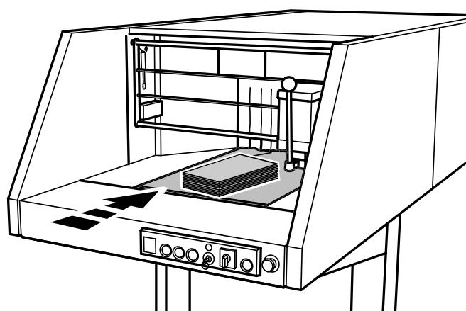
When large amounts of paper are inserted the machine automatically adjusts to a more powerful, slower capacity.
