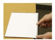
Moving thumb gently along top of wire, sliding hand down binding edge should easily guide all wire fingers into holes. Make sure that all wire fingers go in all punched holes, and turn coil so that fingers reach completely through book.
