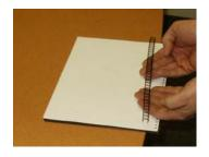
Put punched sheets together into a complete book (also take out the bottom page and place it on the top- see below) with punched edge facing you. Prepare a wire element.
