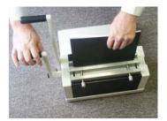
Hold book together and lift with binding edge (and binding wire) pointed downward. Wire should rest easily and naturally in punched holes. Lower the binding edge (and wire) into wire closure mechanism, placing wire down onto steel surface, and close binding handle to close wire. (TitanWire machine showed)
