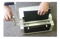
Hold book together and lift with binding edge (and binding wire) pointed downward. Wire should rest easily and naturally in punched holes. Lower the binding edge (and wire) into wire closure mechanism, placing wire down onto steel surface, and close binding handle to close wire.
