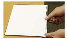
Moving thumb gently along top of wire, sliding hand down binding edge should easily guide all wire fingers into holes. Make sure that all wire fingers go in all punched holes, and turn coil so that fingers reach completely through book.
