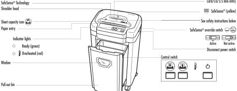
Breakthrough Safety Technology! SafeSense® stops shredding when hands are too close to the opening.
