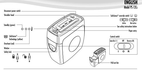
Breakthrough Safety Technology! SafeSense® stops shredding when hands are too close to the opening.
