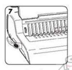
7. Ensure the comb-opening lever is pushed backwards.
