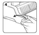
When all punched sheets are loaded onto the comb, push the comb lever backwards to close the comb and remove the bound document.
