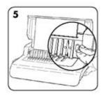
5. Test punch scrap sheets to check edge guide setting.
