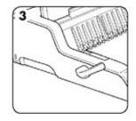
3. Load punched sheets directly onto the opened comb. Starting with the front of the document.
