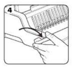
Pull comb-opening lever forward to open the comb.
