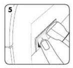
5. Switch the machine on (located at the rear of the machine)
