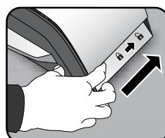
To open the top cover, move the levers on each side of the machine backwards to release the electronic safety catch.
