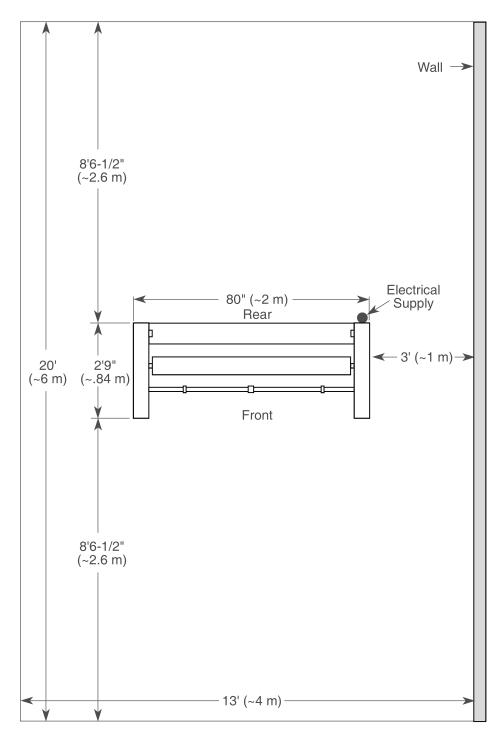
Figure 2-1: Heat Press Space Requirements
