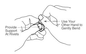
Figure 4-1: Adjusting the Thermocouple
