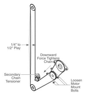
Figure 4-5: Adjusting the Chain Tension
