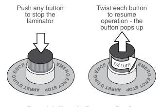
Figure 1-1: Using the Emergency Stop Buttons
