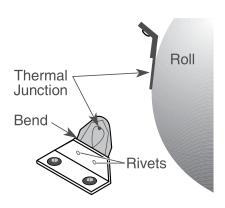
Figure 4-2: Correct Thermocouple Contact
