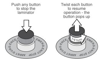
Figure 3-1: Using the Emergency Stop Buttons
