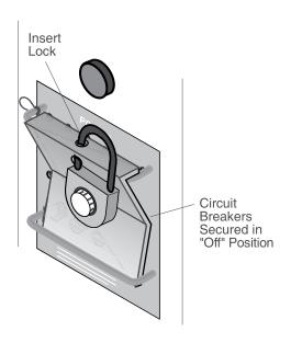
Figure 1-3: Power Lockout
