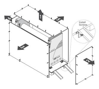
Figure 2-2: Removing the Crate
