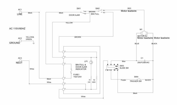
950S/955X 115VAC 60Hz Wiring Schematic
