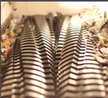
Cutting unit stage 2: downstream shredder
