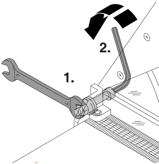
**GB** The machine has a **friction device** on the knife carrier. This insures, that the knife carrier cannot move down on its own. If it does re-adjust the friction device as follows:
