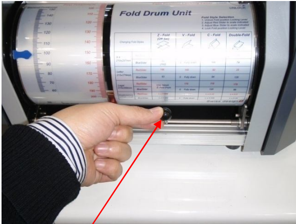
Folding Drum handle in the Unlock(down) position
