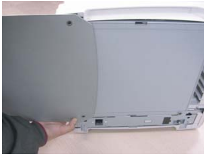
Attach the plate to the foot of the printer.
