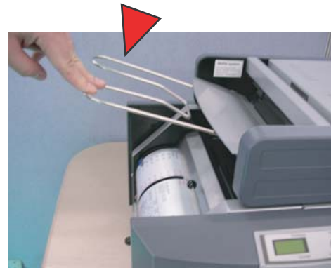
Make sure that the upper tray guide wires are pointing downward.
