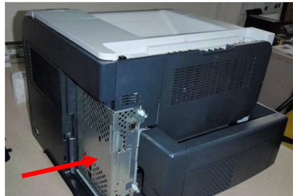
Remove the front communication cover as shown
