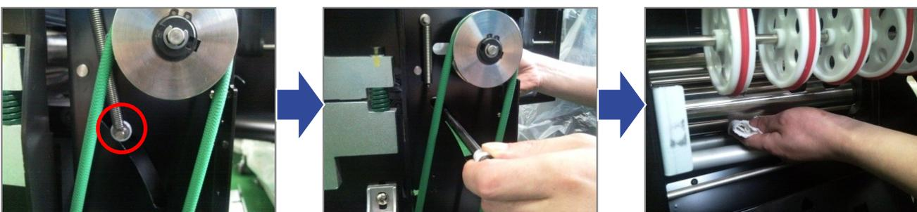
3) Separate the hook and shaft. (Both Side)
