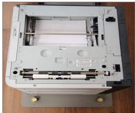
Load the printer onto the printer base plate and adjust the height using the 2 height adjustment bolts. Please note you will require an adjustable spanner for this task
