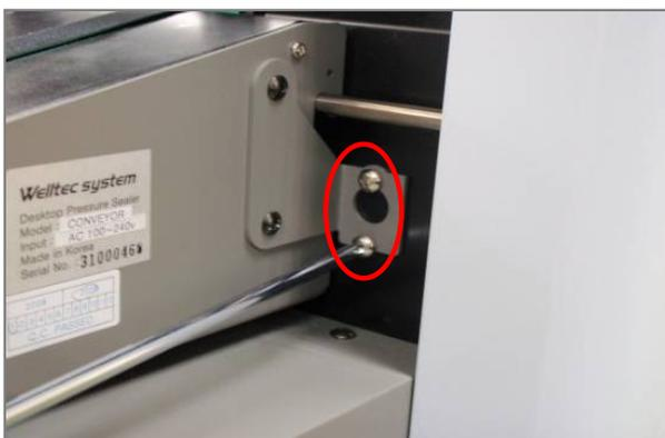
Fix the conveyor as shown with M4 screws supplied
