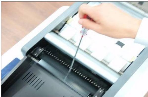
Screw the lower security cover onto the interface with screws supplied
