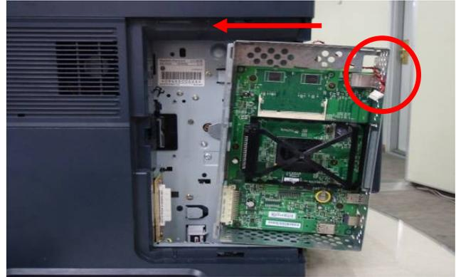
Reassemble the control board
