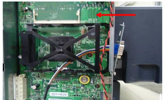
Install the D-Sub Ass'y as shown
