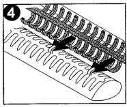
4. Raise the ProClick closing arm. Position the ProClick spine underneath the holding fingers in the top loading area.
