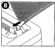
8. To reopen the spine for making edits, position the arm in the downward position. Insert the ProClick spine into the opening tool and slide towards you (the spine opening must be facing downwards).
