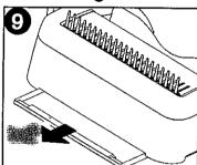
9. Empty the chip tray located on the backside of the machine after repeated use.
