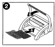
2. Align sheets or covers and insert edge to be bound into punch throat (A). document flush against edge guide and back of punch throat. To punch, handle (B) towards the front of the machine and down.
