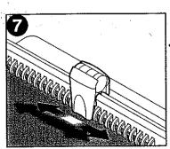
7. Slide the closing tool across left to right to completely close the spine. Raise the arm and release the document from the holding fingers.
