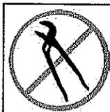
DO NOT USE TOOLS TO LOOSEN OR TIGHTEN TELESCOPING LEGS.
