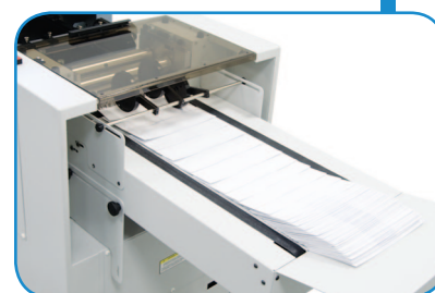
24" outfeed conveyor helps keep forms in a neat order after processing
