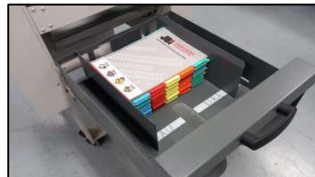
Retractable reception allowing easy handling of punched sheets
