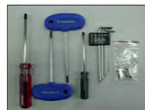
Maintenance tools: 1. Cross-head and flat-head screwdriver - each 1 pc 2. T-type hex wrench (2.5,3) - each 1 pc 3. Hex wrench (1.5/2/2.5/3/4) - each 1 pc 4. Fuse (7A) - 5 pcs
