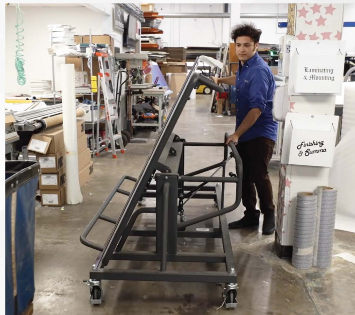
One operator can move 500 lbs. of rigid substrates from warehouse to printing to finishing with minimal effort. Shops have so much equipment in a limited amount of floor space. These tables revert to a 3-ft-wide space.
