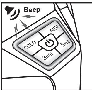
3. During laminator warm-up, the light on the selected thermal mode will flash. Once the appropriate laminating temperature is reached, the 3 beep audible alert will sound. The laminator is now ready.
