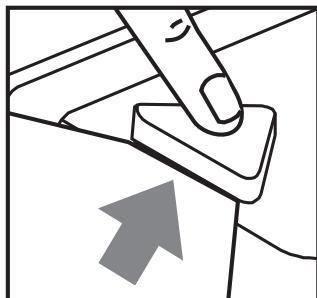
1. Insert the squared corner of laminated item into corner punch slot and press down on punch button.
