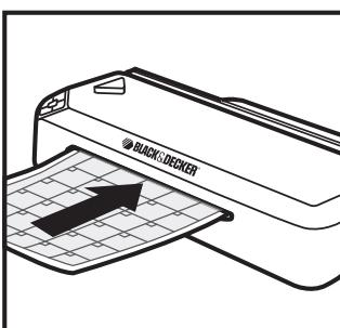
**3.** Insert the sealed end of the pouch straight into the in-feed slot and gently guide forward until the machine pulls it through.
