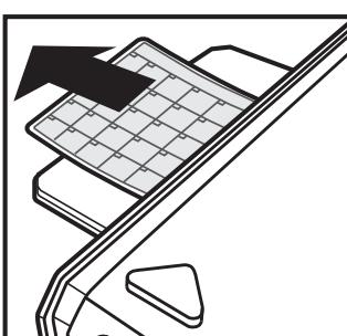
**4.** The pouch will automatically feed through the laminator and exit through the rear. You can remove the laminated item once it has stopped moving.
