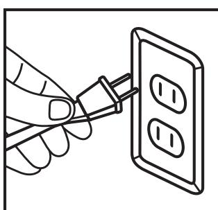
3. Plug the power cord into a standard 120 V outlet.
