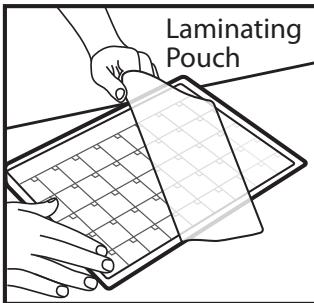
**2.** Center your item in the open pouch, with the top edge of your item towards the sealed seam of the pouch. Ensure there's a minimum border of 1/8" on all sides of the item.
