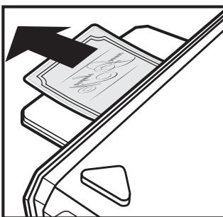
5. The pouch will automatically feed through the laminator and exit through the rear. Allow the laminated item to lay flat during cooling for a more professional appearance.
