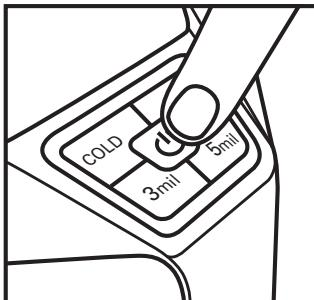
**1.** Turn the laminator on by pressing the power button on the control panel. The unit will automatically start in cold mode, with the COLD button steadily lit.
