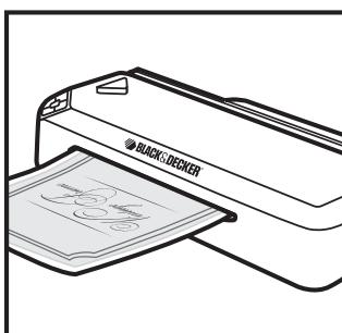
4. Insert the sealed end of the pouch straight into the in-feed slot and gently guide forward until the machine pulls it through.
