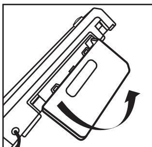
2. Locate the out-feed table, which is stored underneath the laminator (certain models only). Fold open the table to its most upright position.
