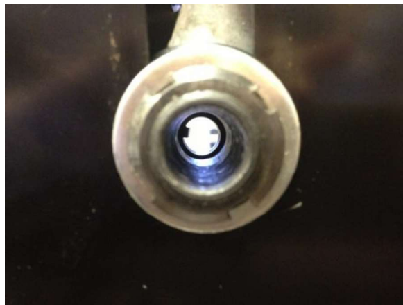
Figure 26. Take note of the alignment groove in the axis hole.
