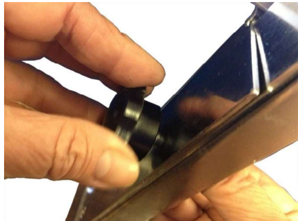
Figure 30. Tighten screw and knob on both sides under the conveyor to lock conveyor in place.
