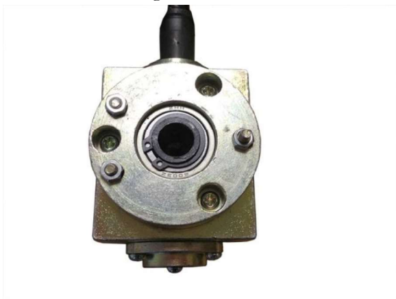
Figure 23. Remove the three screws and nuts on the umbrella gear.
