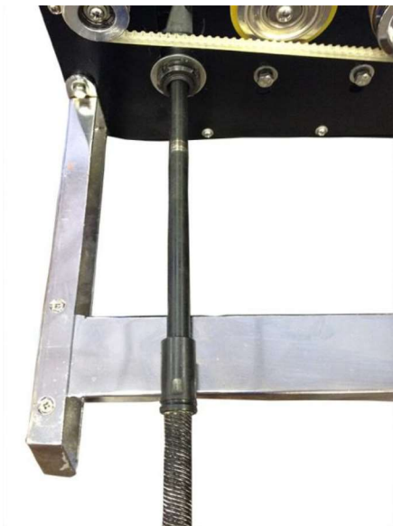
Figure 25. Insert umbrella gear into the axis hole.
