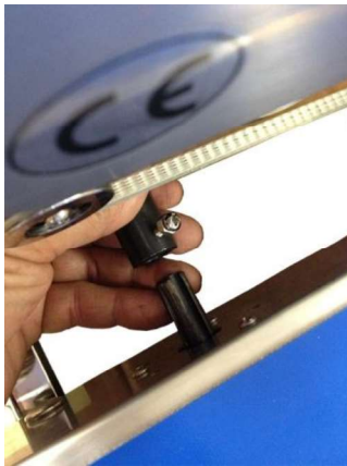
Figure 6. Insert the conveyor middle post in drive shaft. Make sure grooves are aligned.
