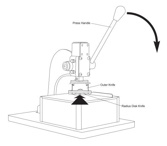
**Note:** Inspect the quality of the cut. The radius on the product should come to an almost perfect blend against the straight edges. The edges of the cut may have a small burr. This burr should not be excessive. If this burr is excessive, the Outer Knife may need adjusting, sharpening, or replacement. (See Page 06)
