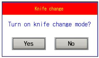
Confirm and make a cut to put the knife into the lower position.
