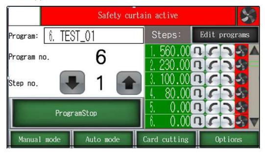
After each cut h\Y backgauge moves to h\Y next step. When h\Y last cut is made in selected program h\Y backgauge automatically moves VUW to step 1 and program can be repeated.
