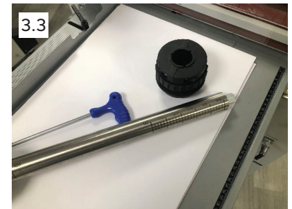
3. Remove film mandrel of the system and loosen the core collar using the blue 5mm Allen key provided
