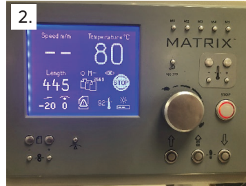
2. Set paper length (exclude the desired overlap). Set temperature to 80°C
