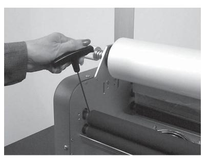
**Shut the machine off!** Minikote EZs have set screws at both ends of each laminating and pull roller. With the use of a 3/32 hex key, loosen all four set screws on the pull rollers. Cut the plastic between the laminating and pull rollers, grab the loose end and pull. The rollers will rotate freely on the roll shafts and the "wrap-around" will easily unwrap. Tighten all the set screws and rethread the film.
