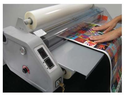
clear the rollers at the end of your document and turn the motor switch to stop. Using the hand held cutter, hold tension on the laminated document and slice through the film to release the document. Multiple documents can be run successfully if desired and cut at a later time.
