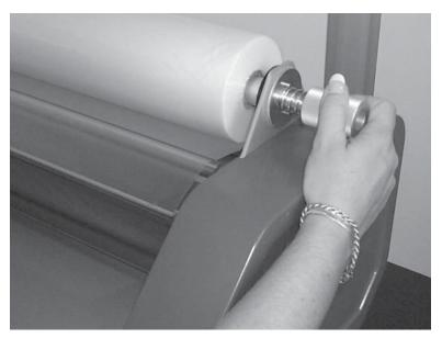
Note: As the diameter of the film roll decreases, tension should be reduced.
