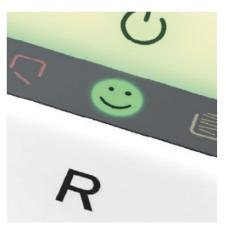
SSC - SMART SHRED CONTROL The smiley has a capacity control function: If it shines green, everything is ok. If the smiley flashes, the shredder has reached its capacity limit.
