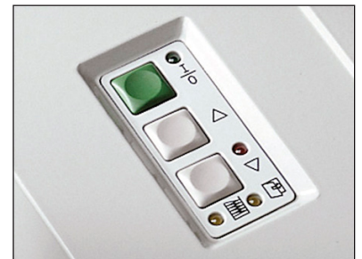
The electronic control panel allows for auto on/off, continuous run, and reverse operation.
