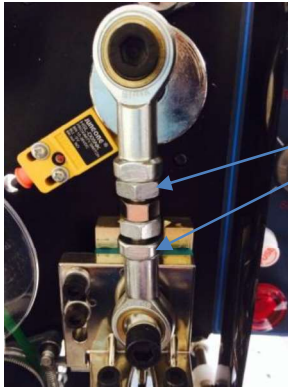
Figure 25. To adjust the length of the connection pole, release either of the two nuts located on the connection pole. Turning the nuts clockwise will cause the connection pole to lengthen. Turning the nuts counterclockwise will cause the connection pole to shorten.
