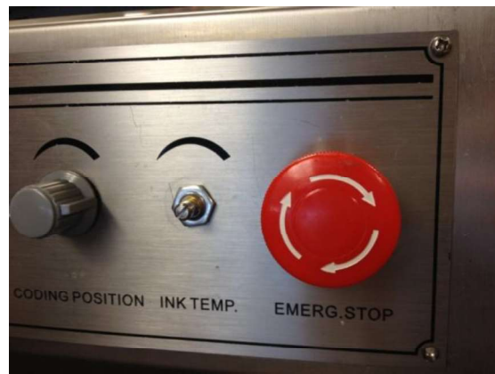
Figure 23. Remove Washer Holding Ink Temperature Potentiometer
