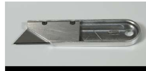
Blade in Blade Magazine with Stiffener
