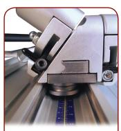
Cutting head is mounted on roller bearings running on steel tracks.
