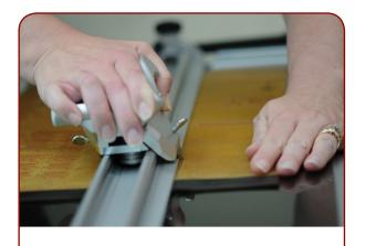
Cutting head is mounted on roller bearings running on steel tracks.
