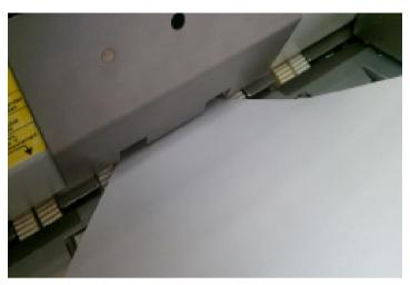
To operate, press **Run** and feed post into hopper tray inside 30 seconds. After this, press Run again.
