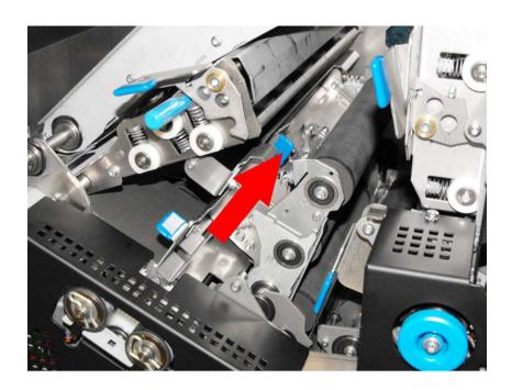
Raise transport assemblies and slide latch inwards to open fold plate 2 for use.
