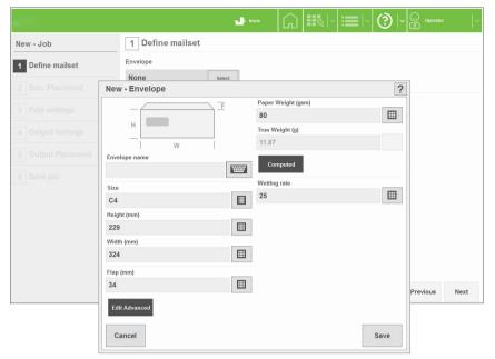
4 Enter the paper weight and envelope weight will automatically calculate, or press **Computed** and enter actual weight.
