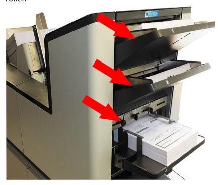
1000-sheet hoppers: slacken knob and use tabs to adjust guides to 1-1.5mm clearance each side.
