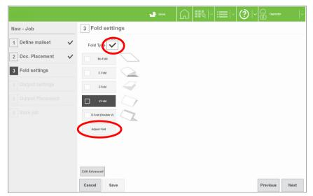
15 The machine automatically selects the optimum fold type. To change this, deselect **Fold Type** and set as required. **Use with caution.**
