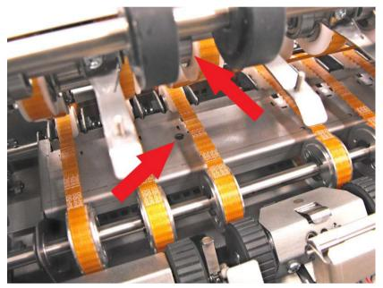
Lower collate clamshell and open upper conveyor (furthest from the envelope hopper) so it locks in place.
