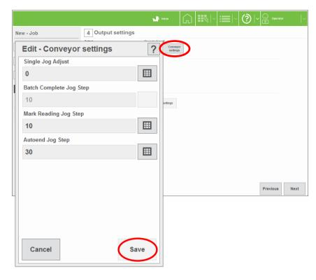
21 If a conveyor is fitted, select **Conveyor Settings** to adjust the Jog function:
