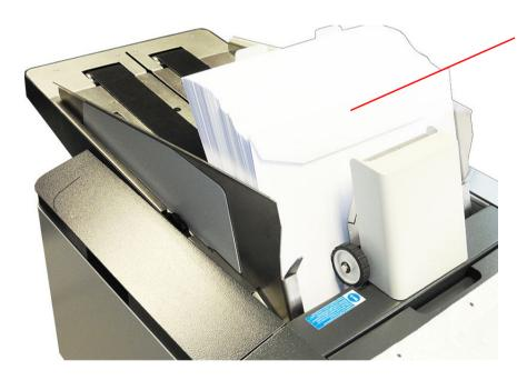
Adjust backrest angle (see below) and load envelopes, flaps forward. Move backrest forward (see below) so envelopes are fully forward, but not tightly packed.
