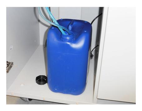
Open the door of the stand below the insert head. Lift the pipes with attached weight out of the bottle.
