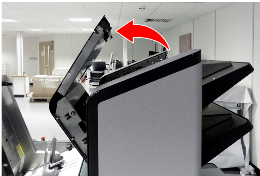
Figure 6.34 - Opening the Tower Folder top cover
