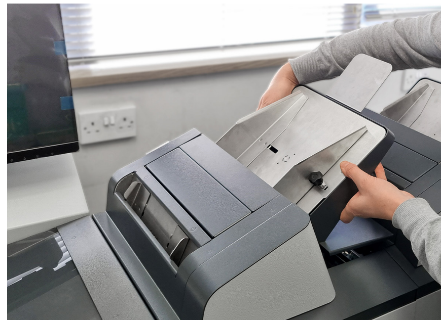
Figure 6.27 - Removing the Feeder Folder hopper tray
