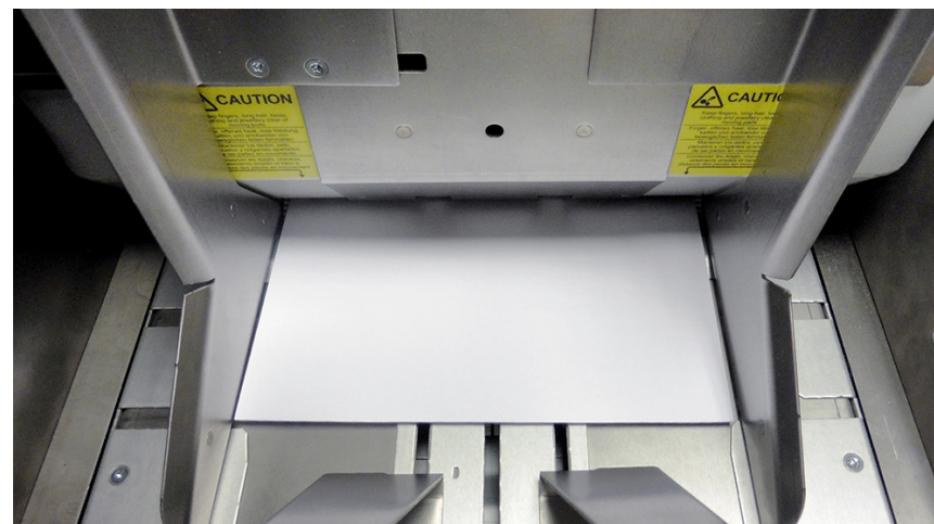
Figure 5.71 – Adjusting the separator gap for Daily Mail - Versatile Feeder
