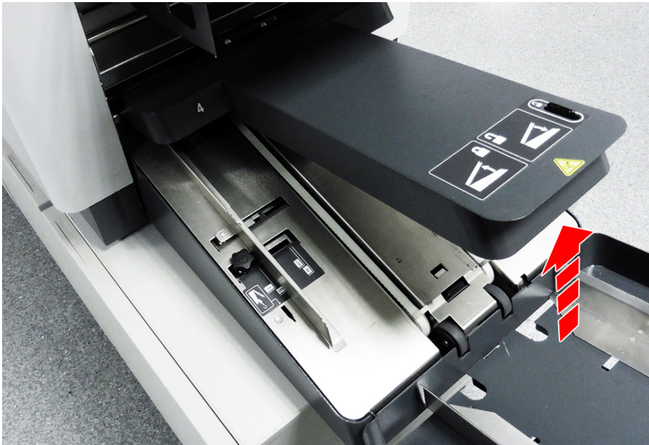
Figure 6.58 – Raising the Accumulator overguide
