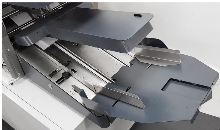
Figure 5.34 - Divert tray attached for Auto feed mode
