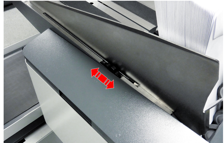
Figure 5.2 – Adjusting the envelope hopper side guides
