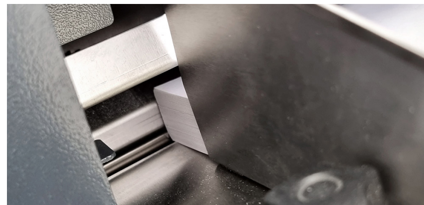
Figure 5.14 - Document leading edges contacting chassis bridge
