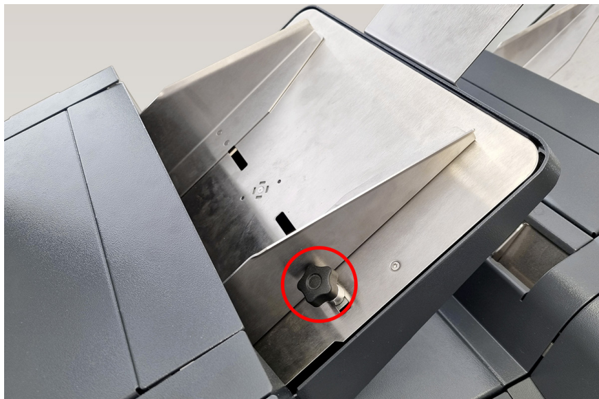
Figure 5.12 - Loosening the Feeder Folder hopper thumb screw knob
