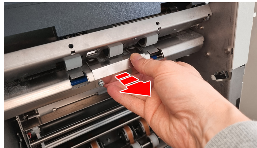
Figure 6.30 - Removing the infeed plate
