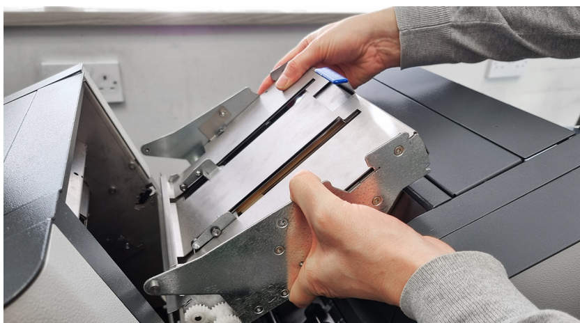
Figure 6.29 - Removing the fold plate assembly
