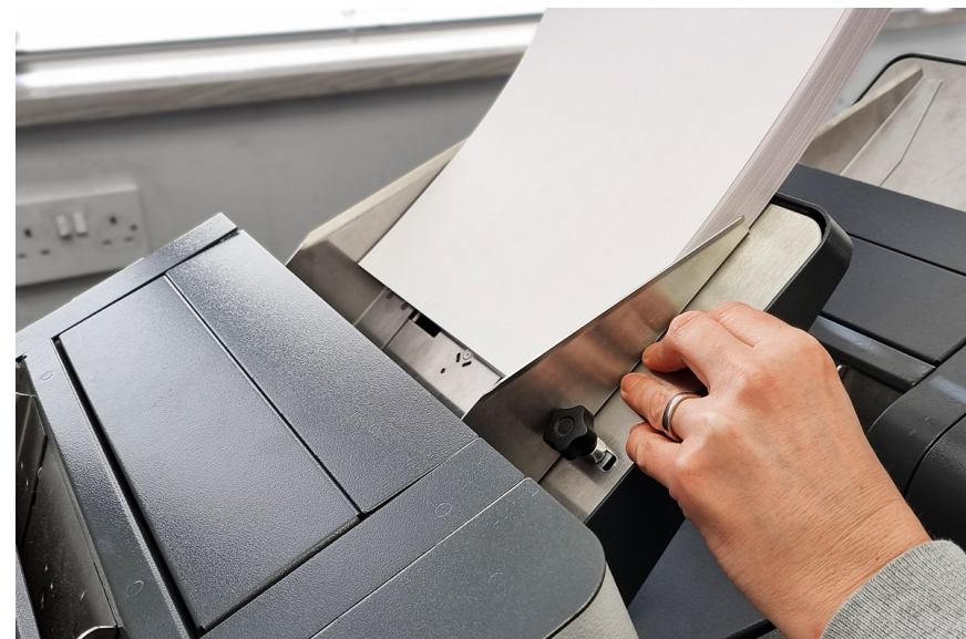
Figure 5.13 - Loading the Feeder Folder hopper
