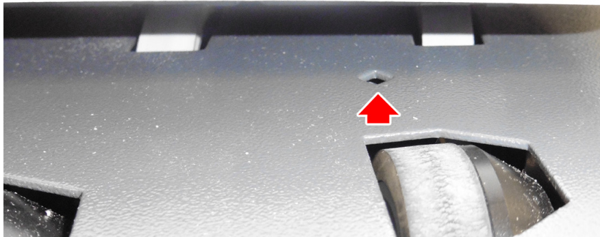
Figure 6.48 – Turn column rotate sensor
