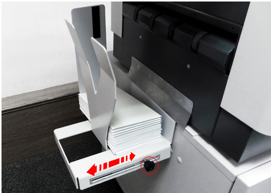
Figure 5.47 – Adjusting the Insert Head catch tray
