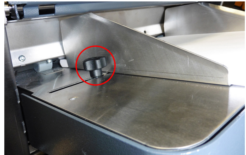
Figure 5.21 – Loosening the 500-Sheet tray thumb screw knob
