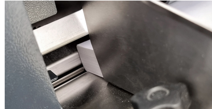
Figure 5.23 - Document leading edges contacting chassis bridge
