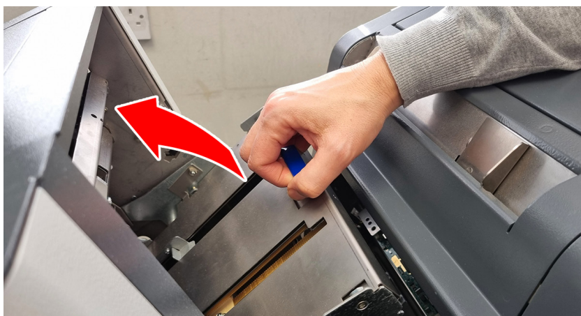
Figure 6.28 - Releasing the fold plate assembly
