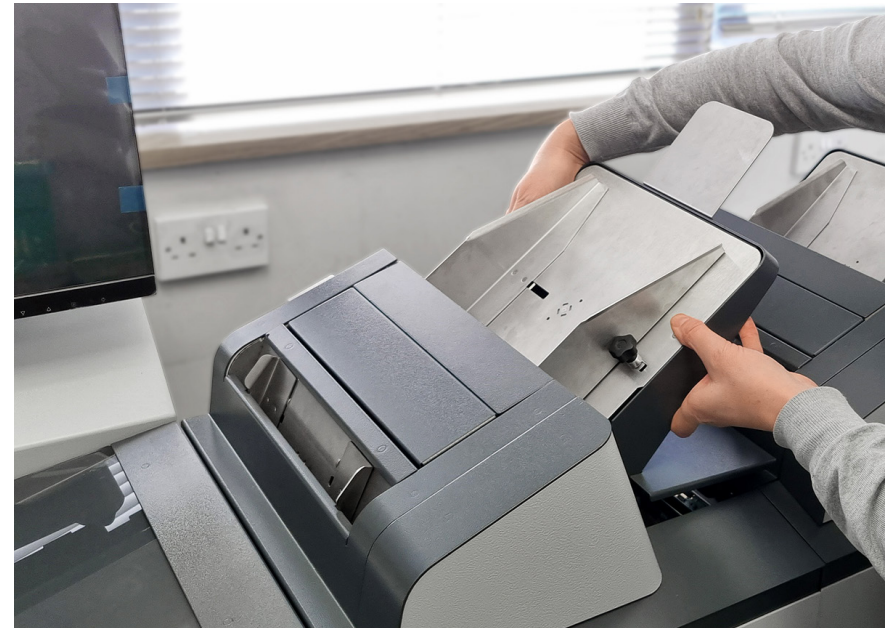
Figure 5.18 - Removing the Feeder Folder hopper tray
