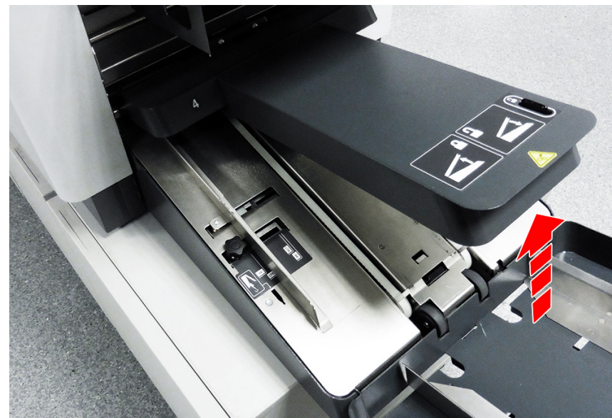
Figure 5.33 – Raising the Accumulator overguide
