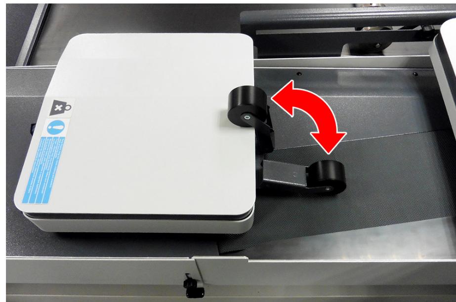
Figure 5.54 - Adjusting the infeed rollers
