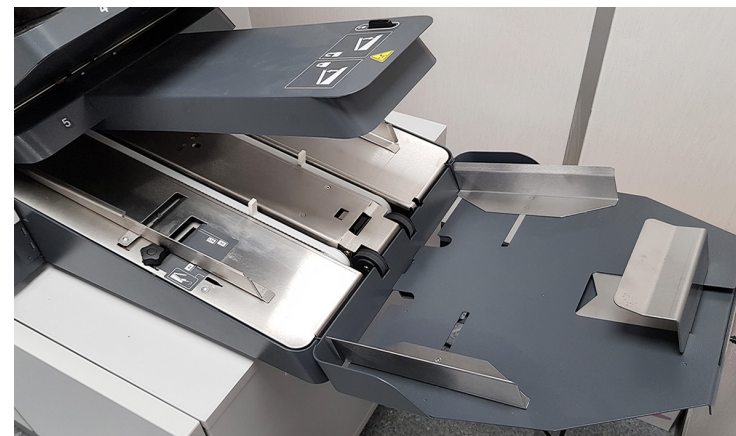
Figure 5.35 - Divert tray attached for Manual feed mode
