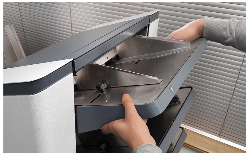
Figure 5.29 - Removing a 500-Sheet tray
