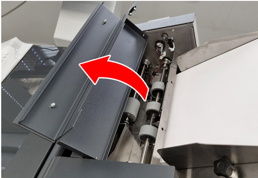
Figure 5.15 - Raising the Feeder Folder top cover showing the grey separator roller
