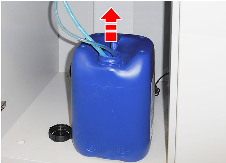
Figure 6.73 – Changing the reservoir bottle
