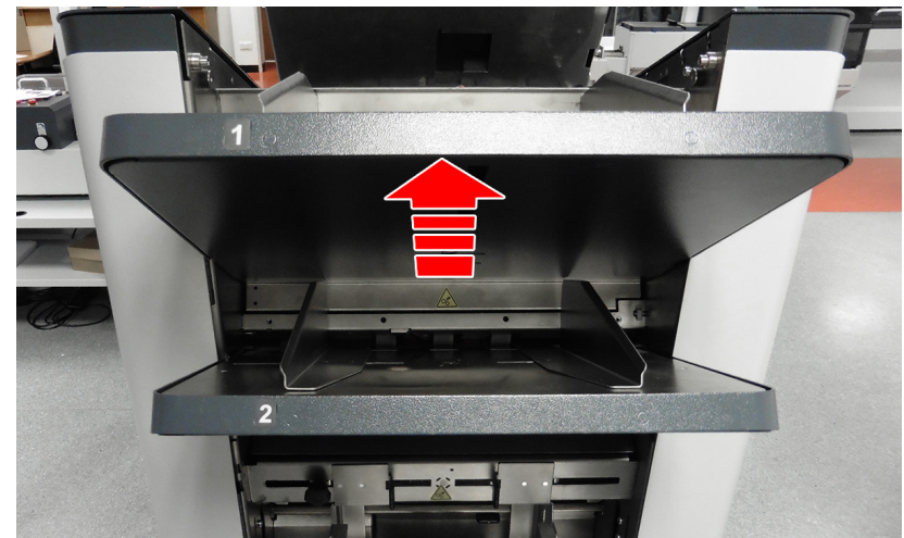
Figure 6.71 - Lifting out the hoppers
