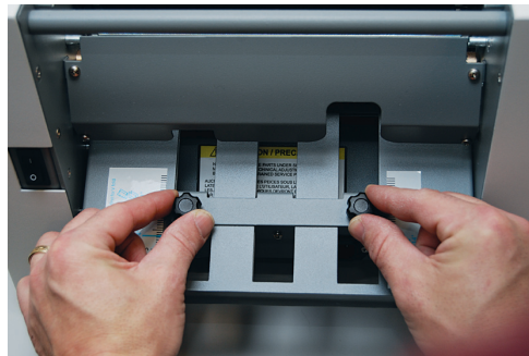
Fig. 2b Adjusting lower fold plate
