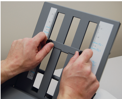
Fig. 2a Adjusting upper fold plate
