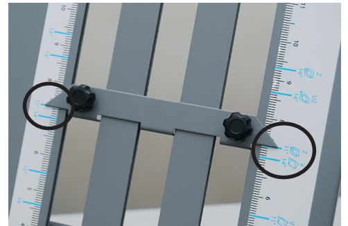
Fig. 2c Setting fold stop
