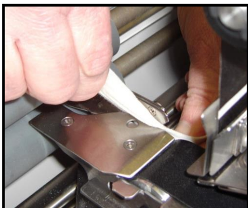
Cleaning the Tab Wrap Guide Located at the exit end of the Right Media Guide Assembly.
