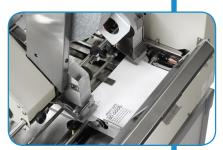
Edge tabbing both sides of a mailpiece simultaneously
