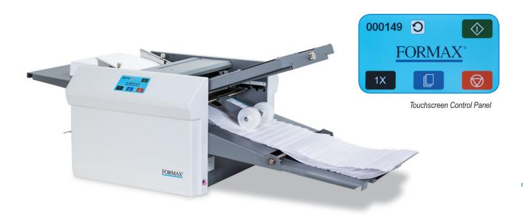
The **FD 346 Document Folder** is a fast, dependable and easy-to-use solution for virtually all folding applications. The *color touchscreen control panel* uses internationally-recognized symbols in place of text, making it easy for anyone to use. Six popular folds are clearly marked on the fold plates: simply slide the fold stop to the desired fold. Additional adjustments can be made with the fine tuning knobs at the end of each fold plate for precision folding.
