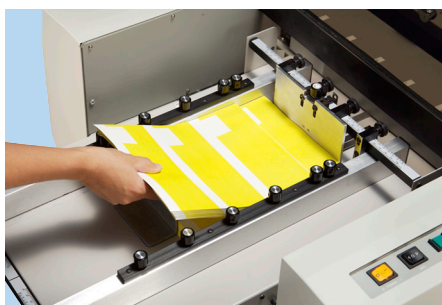
Bottom-feed air system for continuous loading of cut-sheet forms
