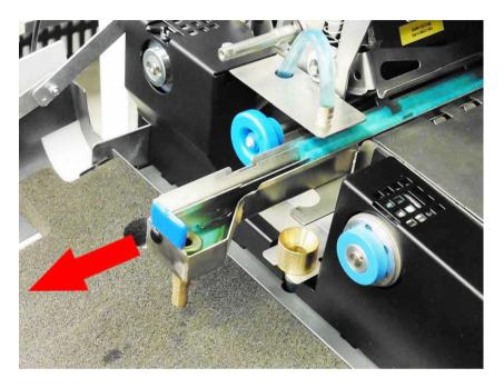
Open the side cover on the insert head. Using the blue tab, lift the end of the wetter tank slightly and withdraw it.
