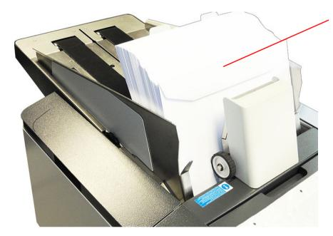
Adjust backrest angle (see below) and load envelopes, flaps forward. Move backrest forward (see below) so envelopes are fully forward, but not tightly packed.
