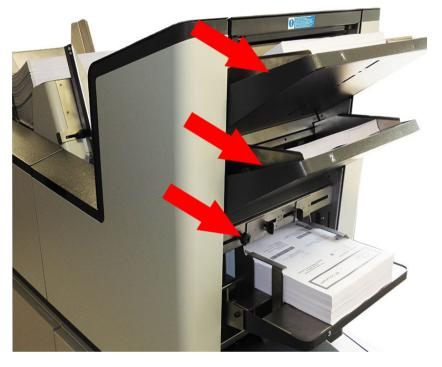
1000-sheet hoppers: slacken knob and use tabs to adjust guides to 1-1.5mm clearance each side.
