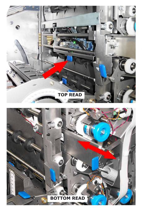
Open side cover and using blue tab, slide CIS reader over to the side of the paper that the label is printed.
