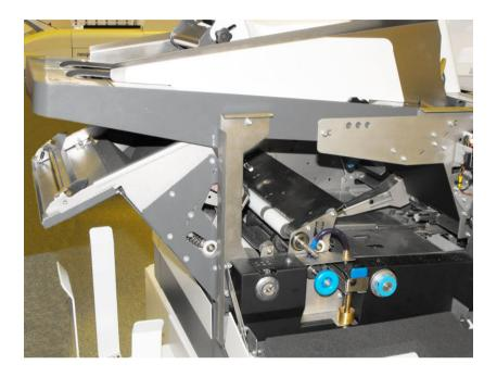
If paper is not fully visible, turn blue knobs to wind into view.
