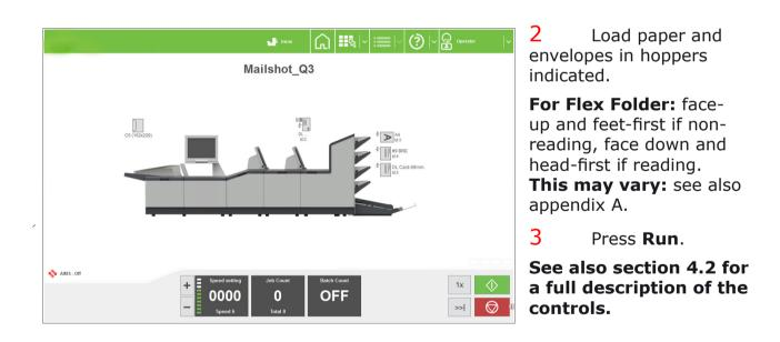
**Important:** If using Cascade, Press **Run** while machine is still running, after reloading the empty hopper. Paper is then fed to pre-load.Otherwise, machine will stop with full hopper: Press **Run** to continue.
