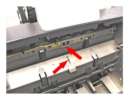
Open perspex top cover and raise collate clamshell (closest to envelope hopper) so it locks in place.
