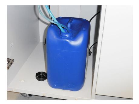
Open the door of the stand below the insert head. Lift the pipes with attached weight out of the bottle.
