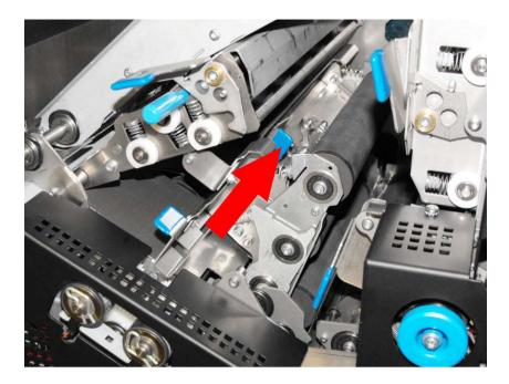
Raise transport assemblies and slide latch inwards to open fold plate 2 for use.
