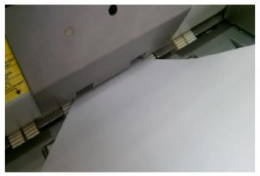
To operate, press **Run** and feed post into hopper tray inside 30 seconds. After this, press Run again.
