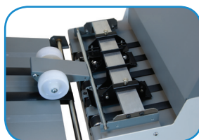
Guide wheels and six-ball-roller deck ensure forms enter the stacker smoothly
