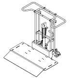
Removable roll ramp permits easily loading rolls.
